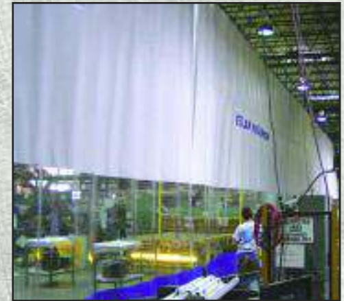
Curtains Separate Wood Working Dust From Window Glass Assembly
